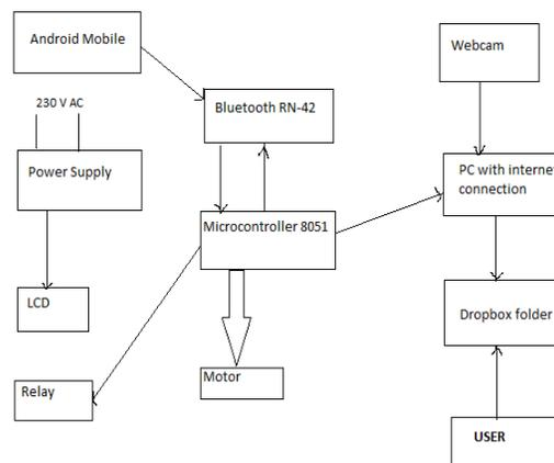
Fig: block diag of automated door lock system
