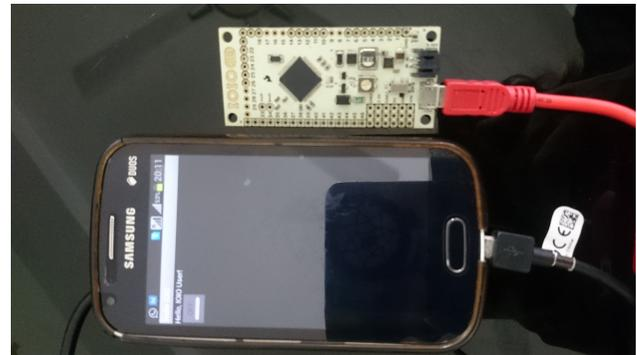
Fig.3 IOIO board interfaced with mobile
