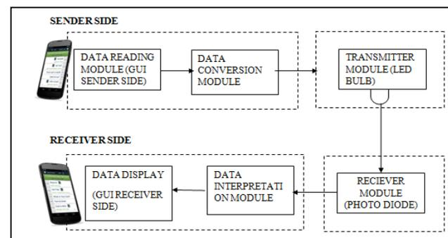
Fig. 1 Architectural Block Diagram
