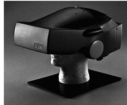
**Fig 1: Head Mounted Display**
