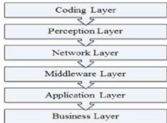
Fig.4. IoT Six Layer Architecture
