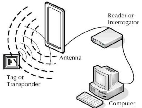
Fig.6. Radio Frequency Identification
