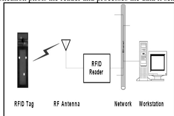
Figure 2. RFID System Components
