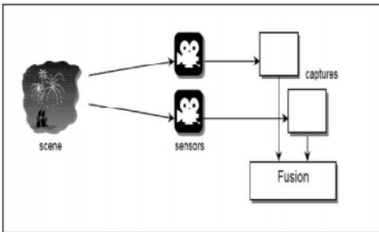
Fig. 2 – Multisensory Image Fusion System
