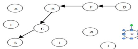
Fig-6: Route Request mechanism in AODV Routing .
